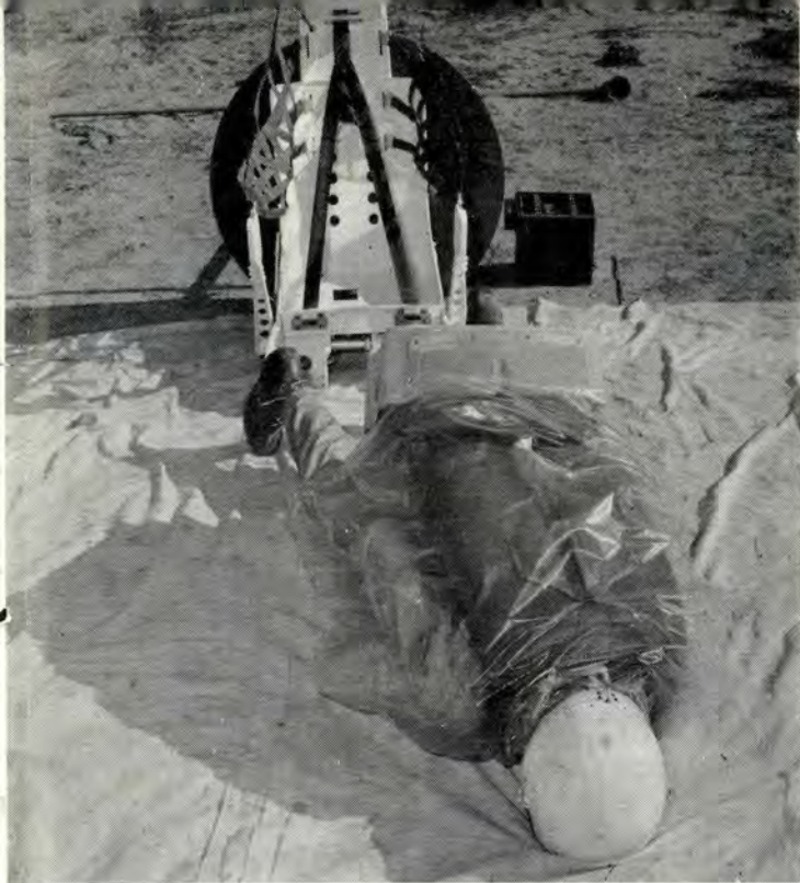
Upper left. The dummy is in the position of a pilot anchored to the seat by G forces and wind pressure after ejection. Upper photo. The power of the butt snapper is graphically illustrated by the distance it throws the dummy from seat. Below. Close-up of seat's features.
